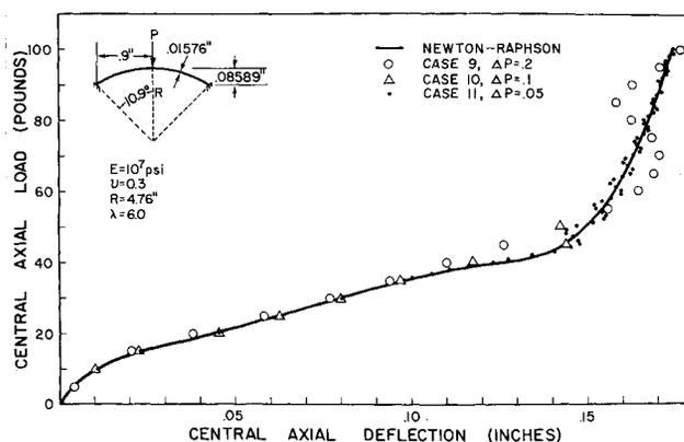
Fig. 2 Load deflection curve for shallow cap.
